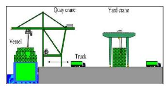
Figure 1: Typical Flow of Containers in Terminal Operations (Ng, 2005)
